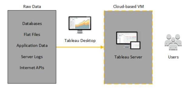
In the following diagram, all of your data is hosted in Microsoft Azure. You can analyze both structured and unstructured data managed in a secure, scalable manner. You may leverage data that resides in Microsoft Azure only, unmanaged data that lives outside of Microsoft Azure, or a combination of both. This flexibility greatly increases the ability of your organization to support moves to the cloud from on-premise data, since both types of data is supported equally.
